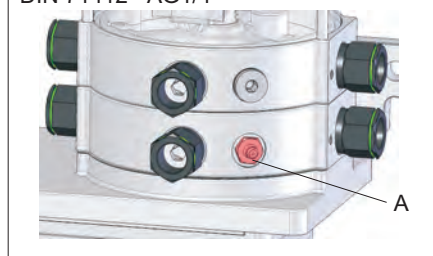
Filling connector "A" Hydraulic-type lubricating nipple DIN 71412 - AG1/4
