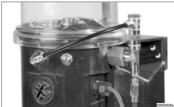
Fig. 13 - Pressure relief valve with grease return
