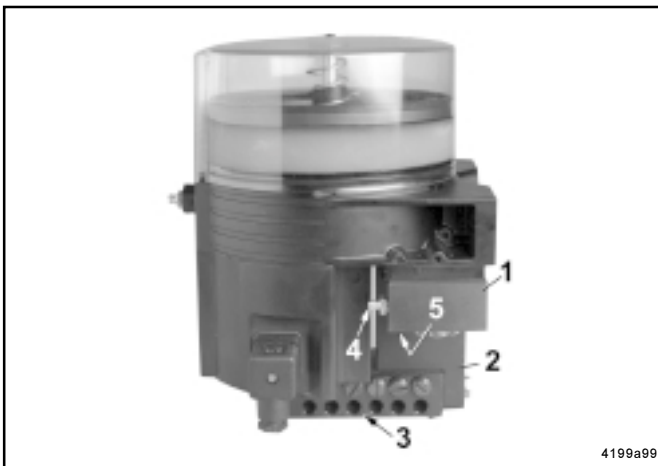
Fig. 17 - QLS 301 with bottom position of the SSV divider block
