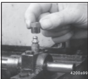
Fig. 5 - Place the Zerk-Lock body over the grease fitting
