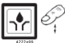
Fig. 31 - Push button for an additional lubrication cycle
