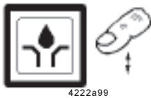
Fig. 21 - Pushbutton for additional lubrication cycle
