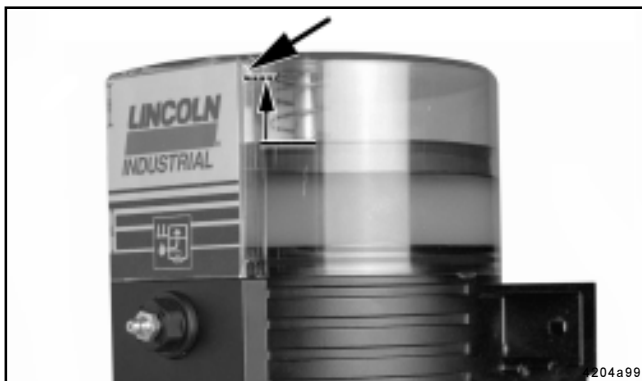
Fig. 10 - Vent hole on reservoir, only for QLS 301
