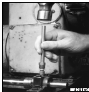
Fig. 6 - Installation of Zerk-Lock body with staking tool
