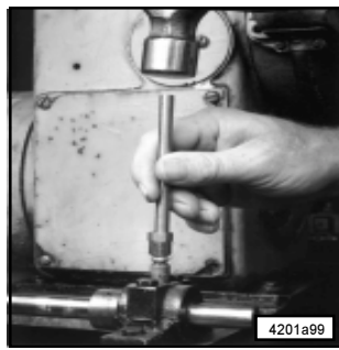
Fig. 6 - Installation of Zerk-Lock body with staking tool
