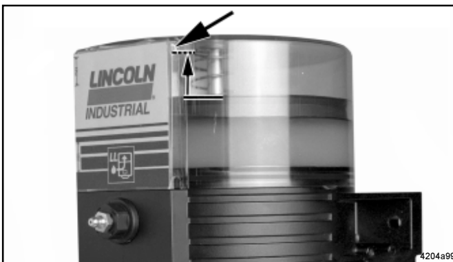
Fig. 10 - Vent hole on reservoir
