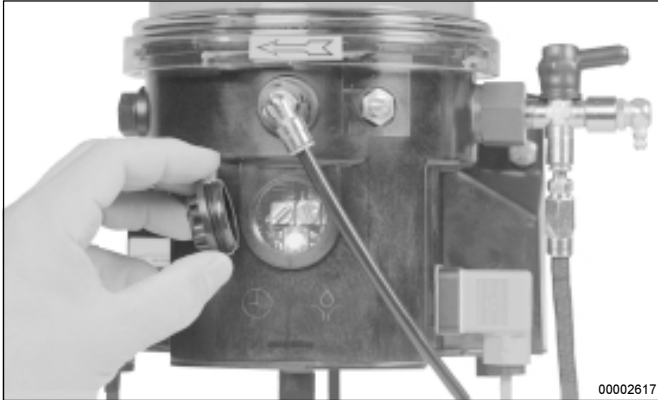
Fig. 7 - The cover to access the printed circuit board has been removed
