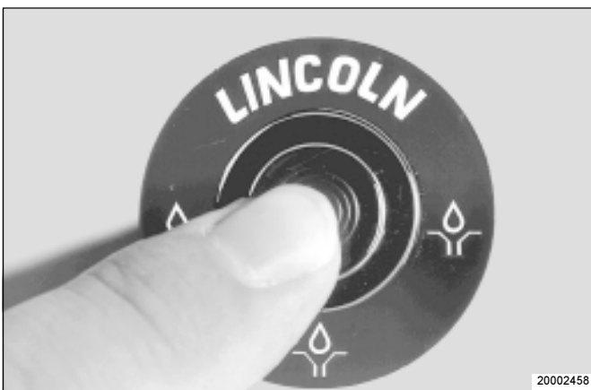
Fig. 13 - To trigger an additional lubrication cycle, only pumps with illuminated pushbutton
