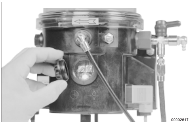
Fig. 17 - The cover to the printed circuit board has been removed
