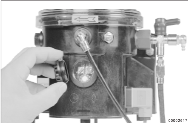
Fig. 7: The cover to the printed circuit board has been removed
