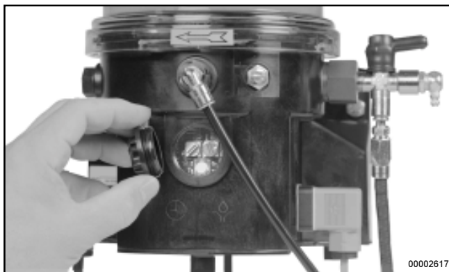
Figure 23- The cover to access the printed circuit board has been removed
