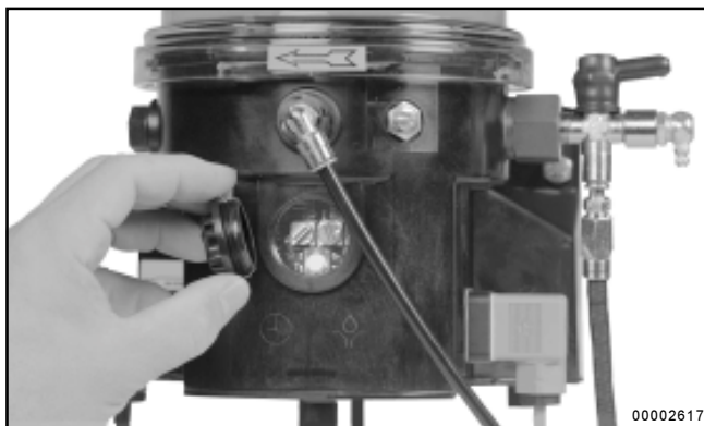
Figure 24- The cover to access the printed circuit board has been removed
