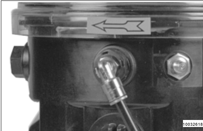
Fig. 17 - Return line connection
