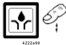
Fig. 25 - Key for triggering an additional lubrication
