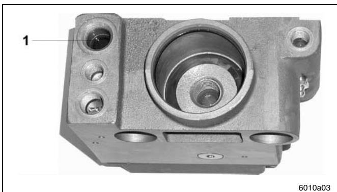
Fig. 10 Cleaning the Oil Strainer
