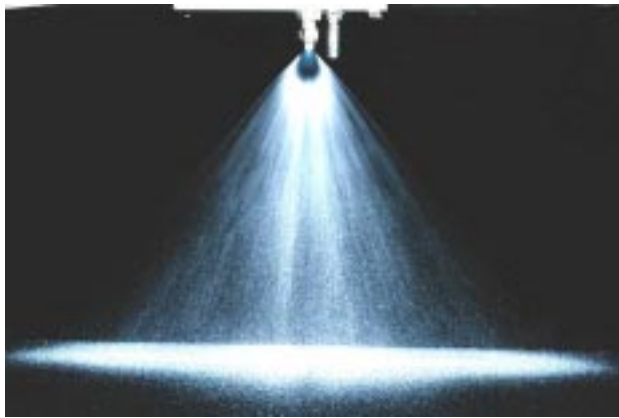
Figure 8: is an actual photograph of the spray pattern produced by the airless spray gear lube system.
