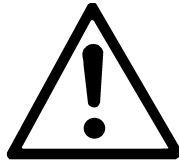
Hazard marking acc. to DIN 4844-W9
