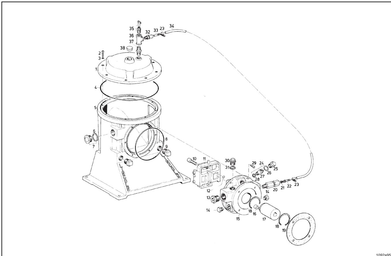
Abb 5.1.1: High-Pressure Central Lubrication pump ZPU 09
