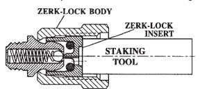
• Place the Zerk-Lock body over the grease fitting and place the staking tool firmly against the Zerk-Lock insert. (Staking tool included in the kit.) Strike the tool sharply with a hammer until the Zerk-Lock insert partially crimps onto the grease fitting.
