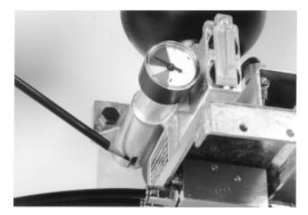
Vent Port Location where grease will discharge when vent screw is opened.
