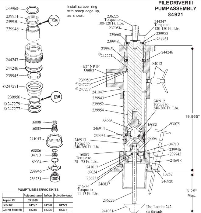
Repair Kit contains all parts needed for complete pumptube rebuild.
