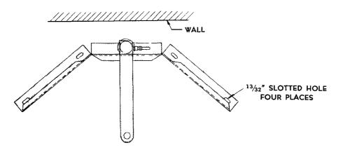
Distance from wall should be sufficient to clear ELEVATOR. Provide a minimum of 30" clearance above PUMPS to permit the vertical lifting of ELEVATOR, for changing drums.
