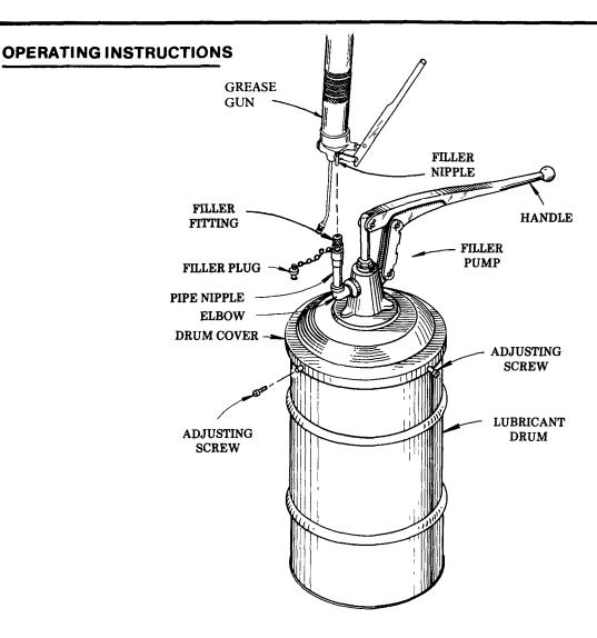
The filler pump is hand operated, designed to lift viscous and semi-solid lubricants from the original drums for loading the containers of the full range of Lincoln grease guns. These grease guns come equipped with a filler nipple for connecting to the outlet of the filler pump, which provides a quick and positive method of filling.
