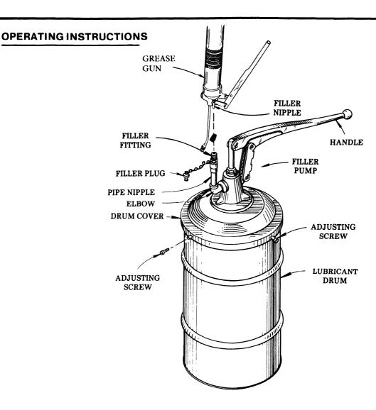
The filler pump is hand operated, designed to lift viscous and semi-solid lubricants from the original drums for loading the containers of the full range of Lincoln grease guns. These grease guns come equipped with a filler nipple for connecting to the outlet of the filler pump, which provides a quick and positive method of filling.
