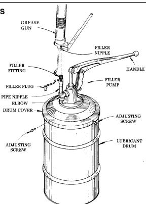
The filler pump is hand operated, designed to lift viscous and semi-solid lubricants from the original drums for loading the containers of the full range of Lincoln grease guns. These grease guns come equipped with a filler nipple for connecting to the outlet of the filler pump, which provides a quick and positive method of filling.
