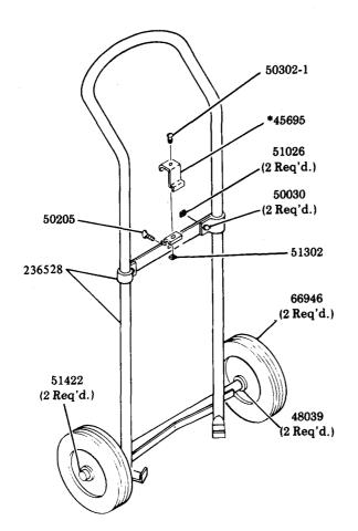
\* NOTE: 45695 & 361040 brackets, 50113 screws and 50754 nuts are used only on Models 346P, 535-58 549-58 and 844.
