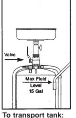
With valve fully open, (Valve handle in vertical position), lower drain bowl to desired height. Always use the tank handle to transport the tank assembly.
