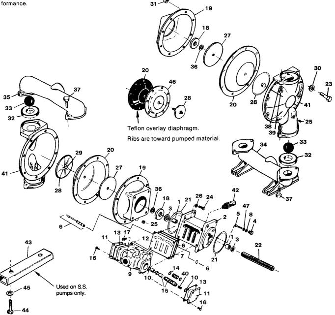
In freezing temperatures the pump must be completely drained when idle. This model must be tilted to allow the liquid from the chambers to run out of the discharge port.
