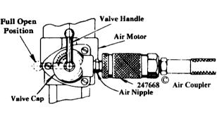
Uncouple 247668 Air Coupler from air nipple. Fill air coupler with No. 10 S.A.E. Motor Oil. Quickly recouple to air nipple. Normal operation of pump will carry the oil to all parts of the air motor which require hubrication.
