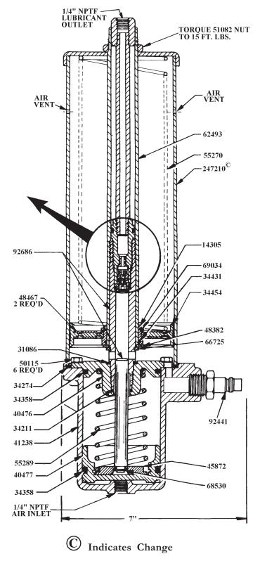
System fails to cycle and calculated system planning has been followed. -- Lubricant may be leaking by the 66250 Ball Check or the 34445 Packing in the 84175 Check and Vent Assembly. Remove these parts and examine for presence of foreign particles. Clean, or replace parts if worn or damaged.
