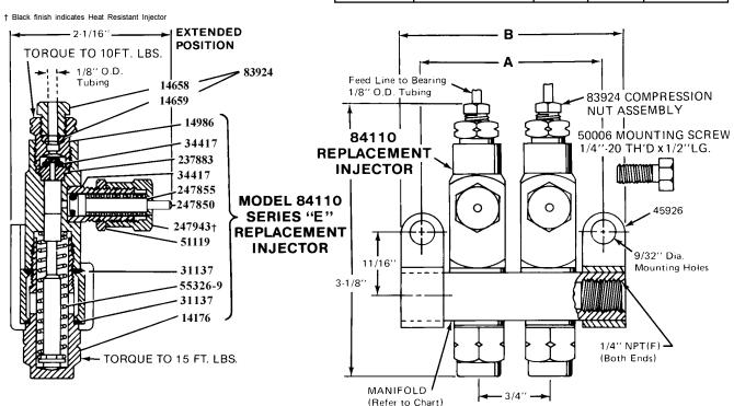
**NOTE:** Injectors from previous series can be improved with stenciled cap and single piece piston by use of 247952 upgrade kit.
