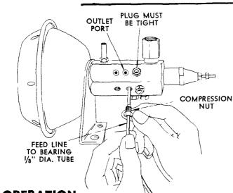
Slide COMPRESSION NUT over FEED LINE. Insert FEED LINE into OUTLET PORT of MULTI-LUBER BODY. Hold FEED LINE securely against STOP in MULTI-LUBER BODY while tightening the COMPRESSION NUT. All FEED LINES must be connected to the MULTI-LUBER before RESERVOIR is installed.
