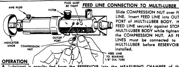
Slide COMPRESSION NUT over FEED LINE. Insert FEED LINE into OUTLET PORT of MULTI-LUBER BODY. Hold FEED LINE securely against STOP in MULTI-LUBER BODY while tightening the COMPRESSION NUT. All FEED LINES must be connected to the MULTI-LUBER before RESERVOIR is installed.
