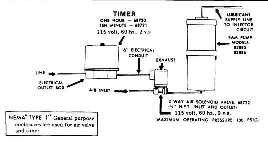
Model 83217 includes ONE HOUR TIMER, 68720 and SOLENOID AIR VALVE, 68722 Model 83218 includes TEN MINUTE TIMER, 68721 and SOLENOID AIR VALVE, 68722
