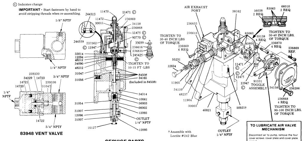
Remove and disassemble the air valve casting from the pump The air valve casting should be cleaned or flushed to remove any chips, or other foreign particles prior to re-assembly Before replacing the toggle assembly, pack
