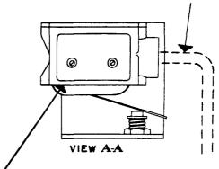
The Switch is a Single Pole Double-Throw Type, which permits wiring it into the Circuit of the Timer and Solenoid Valve. As the Switch is activated by the Low Level Cut-Off, the Switch will shut off the Electrical Current, or it can be wired to Sound an Alarm or Light a Lamp.
