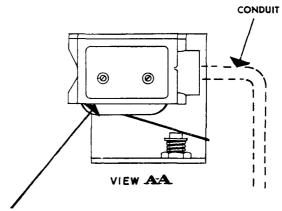
The Switch is a Single Pole Double-Throw Type, which permits wiring it into the Circuit of the Timer and Solenoid Valve. As the Switch is activated by the Low Level Cut-Off, the Switch will shut off the Electrical Current, or it can be wired to Sound an Alarm or Light a Lamp.
