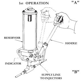
The outward stroke of the Pump Handle forces lubricant into the Supply Line.
