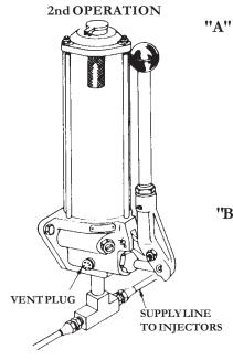
"A" Venting of lubricant pressure in Supply Line.
