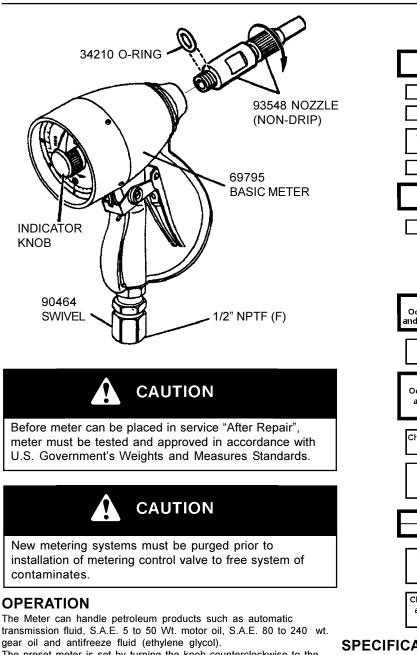
The preset meter is set by turning the knob counterclockwise to the desired amount amount of material to be dispensed. The trigger is then depressed and locked in the "on" position. The pointer knob rotates clockwise towards zero where it strikes a pin in the meter face above the "0" zero, which releases the lock bar automatically stopping the flow.
