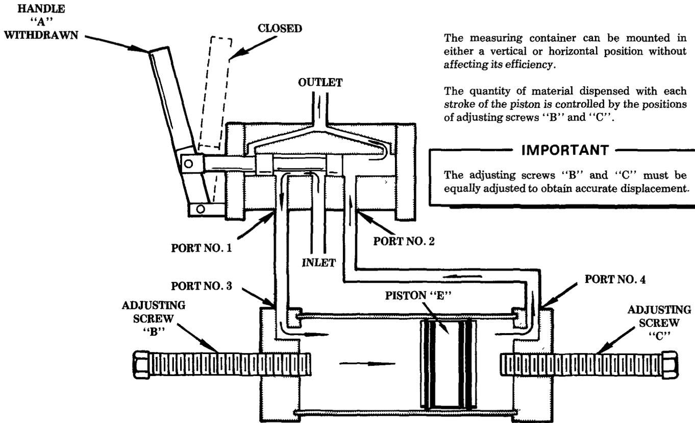
The measuring container can be mounted in either a vertical or horizontal position without affecting its efficiency.
