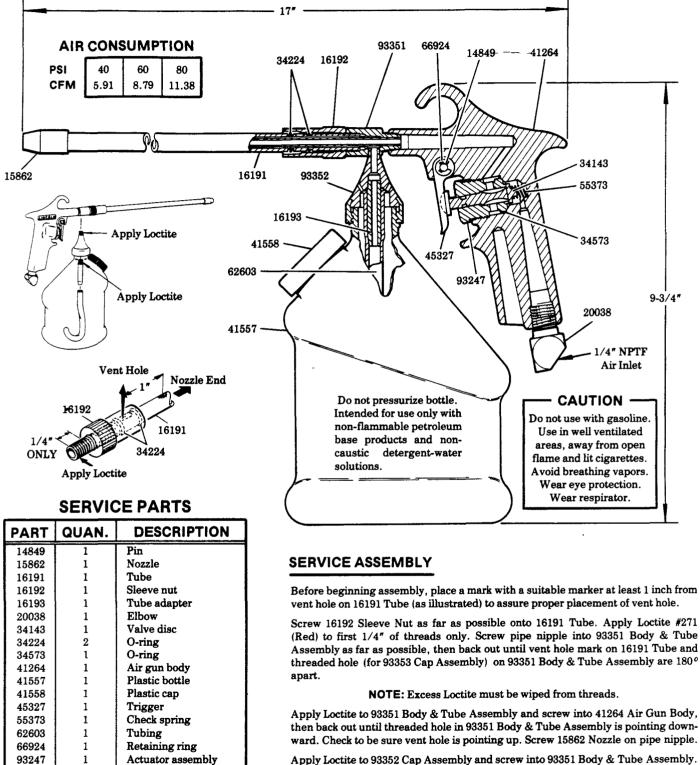
Apply Loctite to 93352 Cap Assembly and screw into 93351 Body & Tube Assembly. Apply Loctite to 16193 Tube Adapter and screw into cap assembly.
