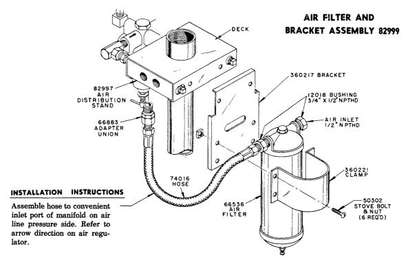
Assemble 360217 Bracket to holes in side flange of the air distribution stand deck. Hold air filter to bracket with clamp. Connect air hose to air distribution stand.
