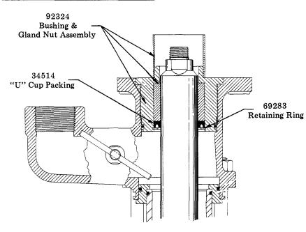
The Teflon Gland and Piston Packing Kit should be used when dispensing materials which are not compatible with the standard Polyurethane and Buna-N Packings
