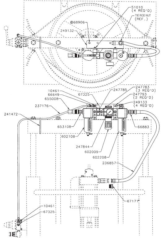
\*Used to adapt 1/2" NPTF(M) on hose to 3/4" NPTF(F) thread, if required.
