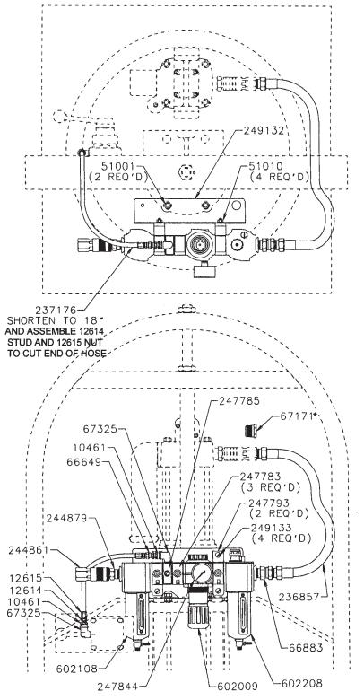
\*Used to adapt 1/2" NPTF(M) on hose to 3/4" NPTF(F) thread, if required.
