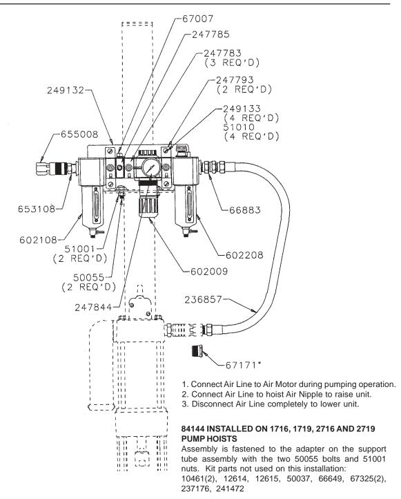
\*Used to adapt 1/2" NPTF(M) on hose to 3/4" NPTF(F) thread, if required.
