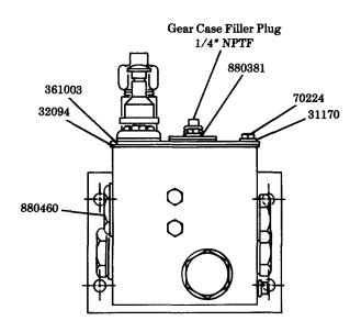
Fill gear case with 90 wt. gear oil. Change every 3 to 6 months.
