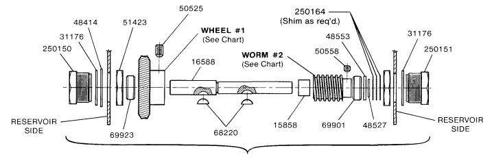
CROSS SHAFT ASSEMBLY DETAIL
