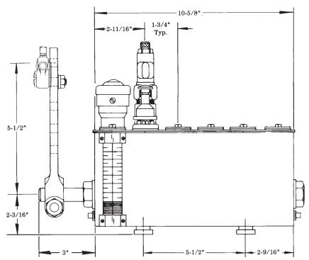
Connecting rod linkage to be supplied by customer.
