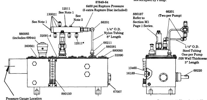
Remove 16189 Plugs & 13465 Nuts for Automatic Oil Level Control.
