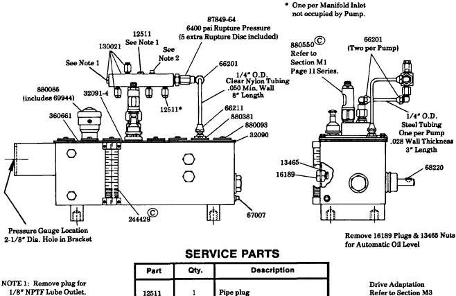
NOTE 1: Remove plug for 1/8" NPTF Lube Outlet. NOTE 2: Remove plug for 1/4" NPTF Lube Outlet.
