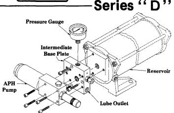
to priming position. Hydraulic pressure from a three-way solenoid valve is connected in Inlet Cylinder #1. APHS pumps can operate at a maximum of 25 strokes per minute with oil, 10 strokes per minute with grease.
