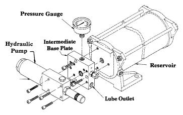
The 87202 single acting pump has one hydraulic connection to power the piston on the delivery stroke. A spring returns the piston to priming position. Hydraulic pressure from a three-way solenoid valve is connected in Inlet Cylinder #1. This pump can operate at a maximum of 25 strokes per minute with oil, 10 strokes per minute with grease.
