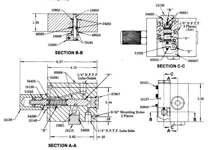
Model 87800 reacts to no-flow conditions in lubricant supply lines by actuating an integral three-way air valve to provide a pneumatic failure signal. In series type lubrication systems the pneumatic no-flow valve is normally installed in the main lubricant supply line between the pump and the master divider valve, eliminating the need for explosion-proof electrical components in hazardous areas.
