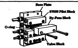
The pilot block, valve blocks and by-pass blocks (if any) are fastened to a base plate mounted on the machine to be lubricated. The base plate contains the divider's inlet and outlet connections, interrelated passageways, and built-in check valves. All piping of lubricant to and from the divider valve is connected to the base plate.
