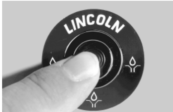
Fig. 11 - To acknowledge a fault
